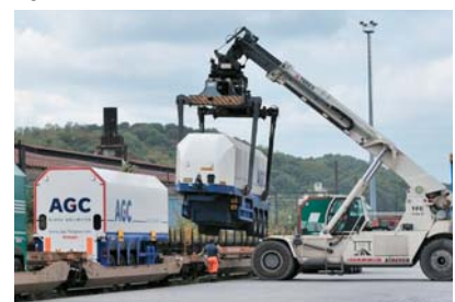
Trailer loaded on a wagon for transportation by rail
