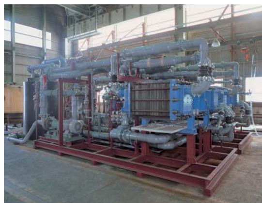
Electrolyzer incorporating the Selemion
