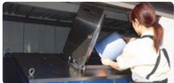
Inputting garbage into the processing machine
