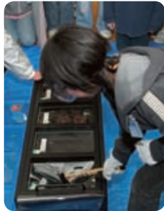
Breaking test conducted to compare the strength of laminated glass for disaster resistance with ordinary glass
