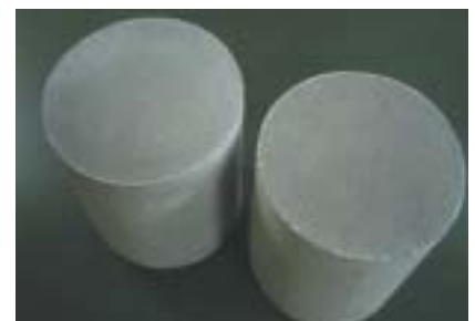
These silicon nitride filters contain around 40 pores/cm 2 . The internal structure resembles a honeycomb
