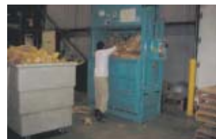
Paper compression machinery for recycling of kraft paper
