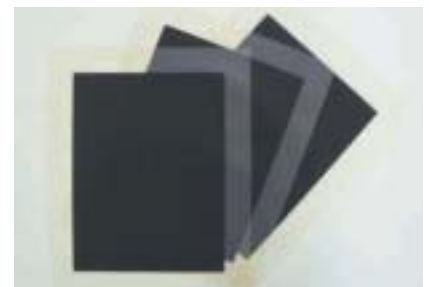
A membrane-electrode assembly (MEA) consists of a proton-exchange membrane and electrodes in a single unit. Sandwiched between separators, these can be packed on top of each other to form a stack. Together with peripheral devices, the stack forms a fuel cell system for clean power generation
