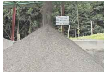
Inorganic slag that can be recycled into a subbase course material
