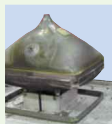
CRT disassembly process at the recycling company
