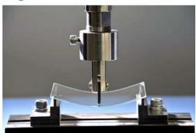
Stress Test (Three-point bending with 1.1 mm-thick glass)
