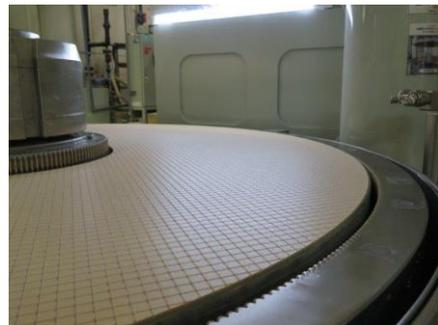
Multiple layers of optical thin films with different refractive rates are deposited to realize various spectroscopic characteristics.
