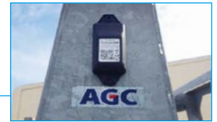
A logistics tracker mounted on a glass pallet
